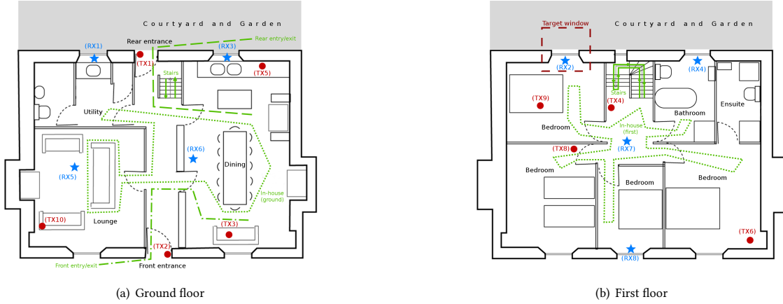
Fig. 20. Approach patterns and equipment placement. The target window of the intruding drone is indicated by a red dashed box. The receiver locations are marked with blue stars, whereas the static transmitter locations are denoted with red dots. Green lines indicate approach patterns.
