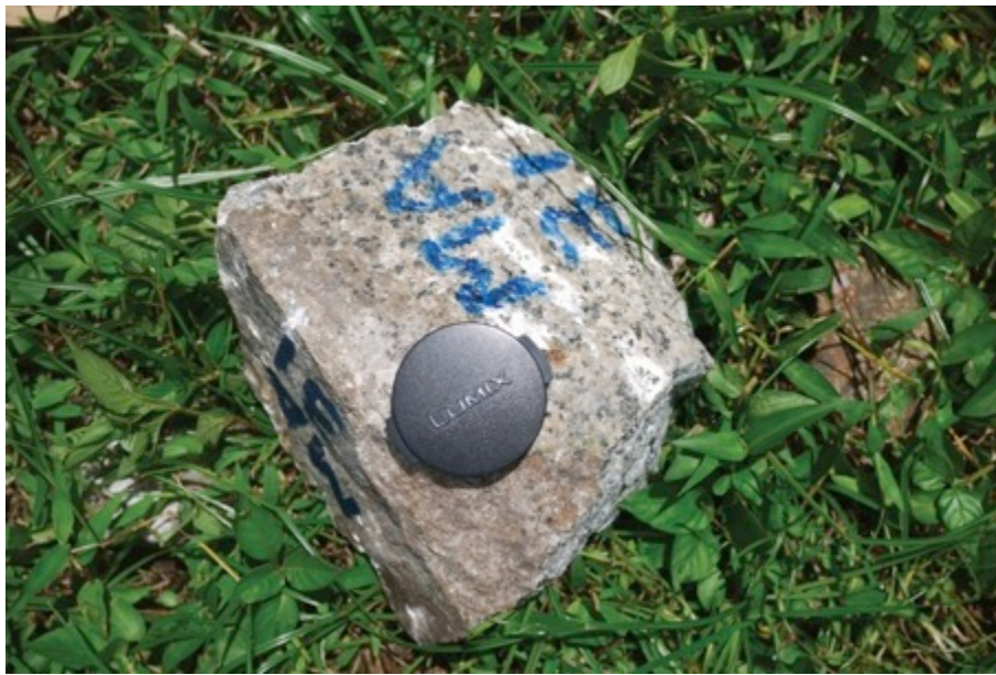
Plate 2.15 Textural variation of Kuala Lumpur granite along the pluton roof-zone boundary can be large, ranging from microgranite to coarse-grained biotite granite. This K-feldspar megacrystic mesogranite (MA31) was collected along the Karak Highway (E8) near Kuala Lumpur.
