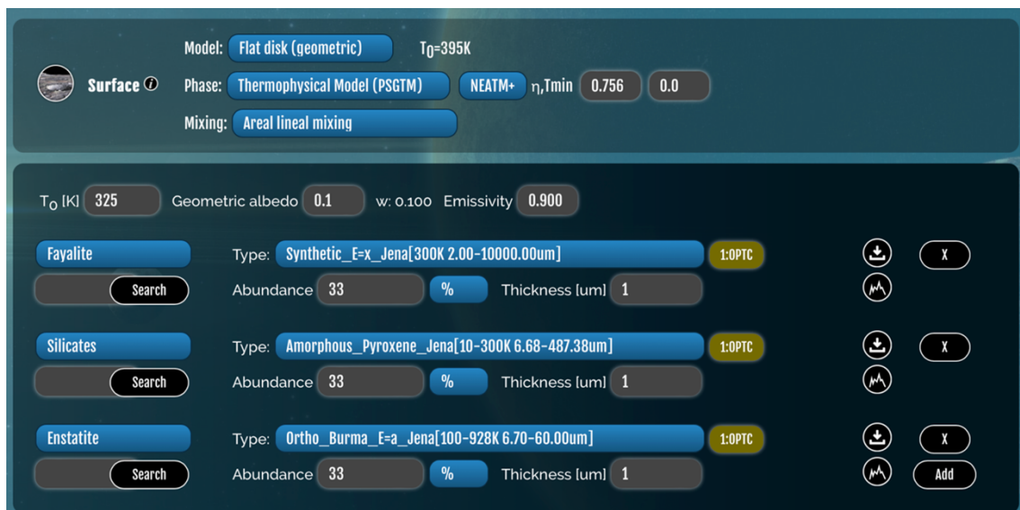
Figure 9-7: The minerals and abundances used in PSG to generate the emission spectrum for the purely rock material surface.
