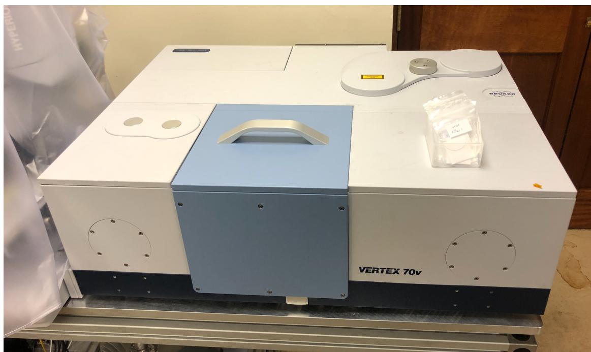
Figure 3-8: Bruker VERTEX 70v Spectrometer, used for all transmission measurements detailed in this chapter.
