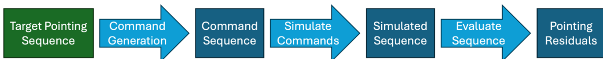
Figure 5-36: the pipeline for evaluating TIRI commanding schedules against the pointing sequence defined by the operations plan.
