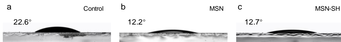
Supplementary Fig. 11. Contact angles of the NBG perovskite precursor solution on (a) PEDOT:PSS-, (b) PEDOT:PSS/MSN-, and (c) PEDOT:PSS/MSN-SH-coated substrates.
