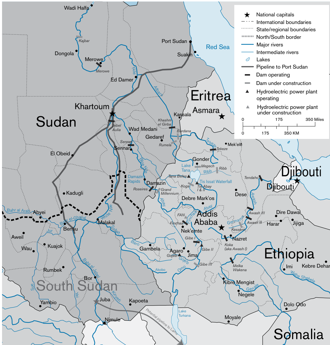
Figure 5.2 Map of Ethiopia and the hydraulic works on the Blue Nile. The Grand Dam is located near the Sudanese border and indicated on this map as the Grand Millennium Dam. Source: (Verhoeven 2011). 109
