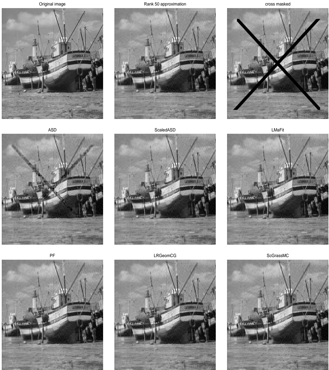
Figure 5.2: Image reconstruction for “Boat” from cross masked. The size of the image is 512 \times 512 . The desired rank is 50, and 6.9% entries of the low rank image are masked in a non-random way.
