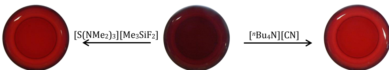
Figure 4.51: Colour change from the dark brown free receptor [VIIXg]I to the red adduct VIIg·X (X = F or CN).
