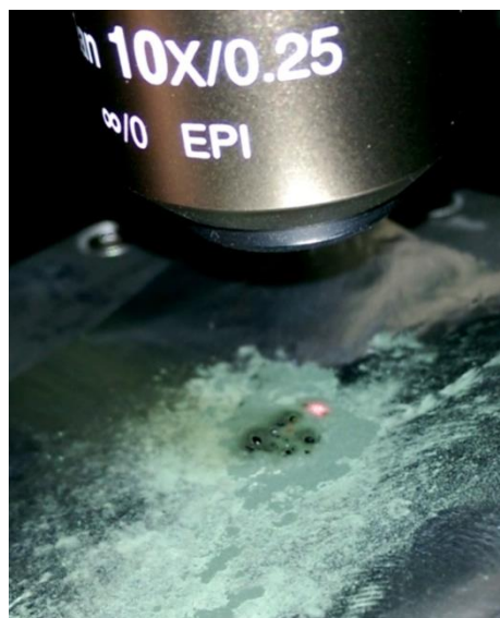
Figure 5.12: Compound X under a 1064 nm laser for attempted solid-state resonance Raman spectroscopy measurements.
