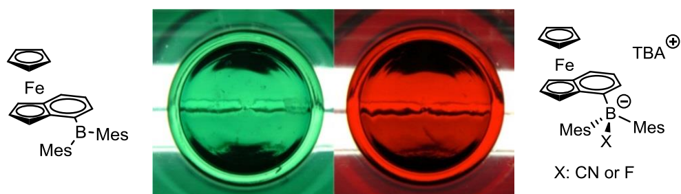
Figure 3.29: (left) sensor IIIe in thf (right) IIIe in the presence of [n\text{Bu}_4\text{N}]\text{F}\cdot 4\text{H}_2\text{O} or [n\text{Bu}_4\text{N}][\text{CN}]\cdot 3\text{H}_2\text{O} in dry thf.
