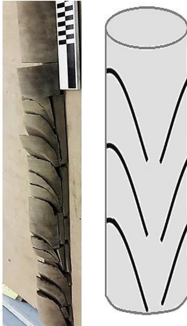
Figure 3.16 Example from the core samples of petal-like fractures induced by drilling.
