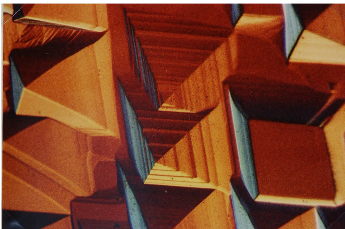
Plate 8. DIC micrograph of a calcite crystal etched in a solution containing 50 mM maleic acid (pH 8.77 - 8.79) and 0.35 M KCl for 12 hours (magnification approximately \times 200 ).
