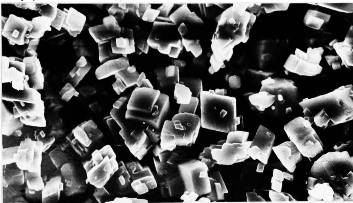
Plate 12. Scanning electron micrograph of calcium carbonate powder. Magnification x2040. (Courtesy of Cookson Technology Centre).
