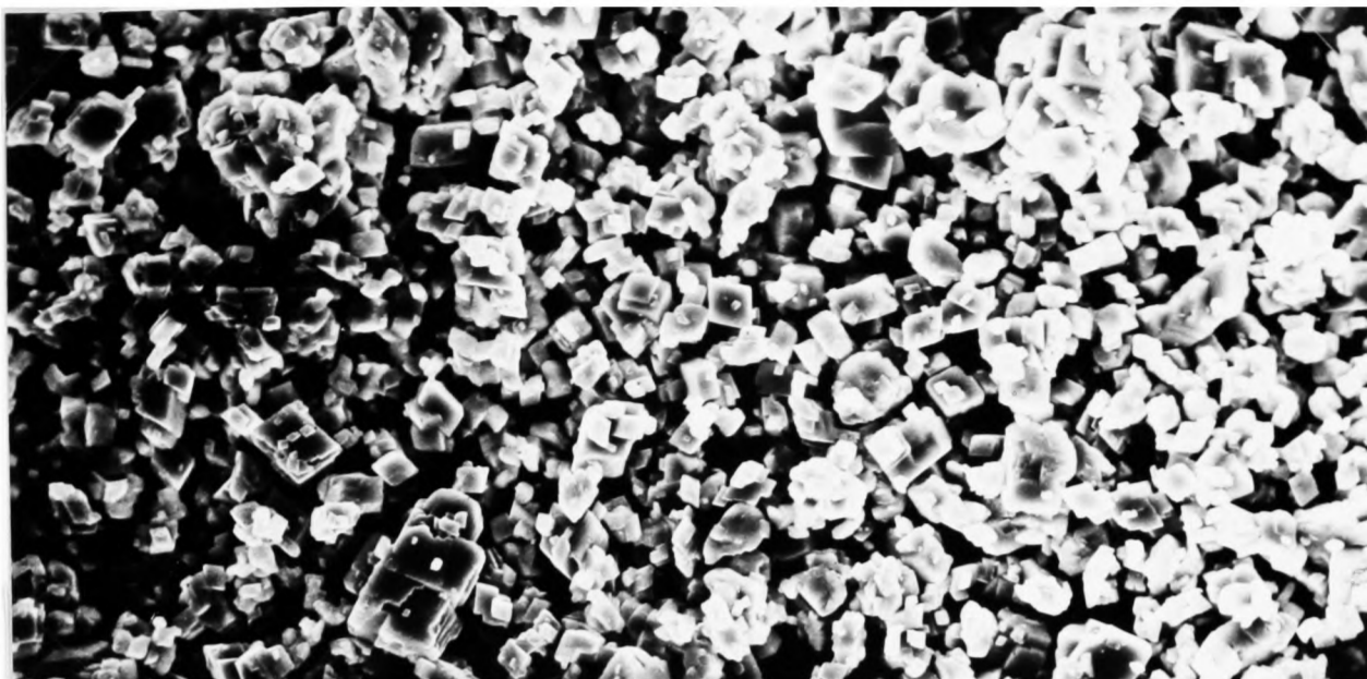
Plate 11. Scanning electron micrograph of calcium carbonate powder. Magnification x628. (Courtesy of Cookson Technology Centre).
