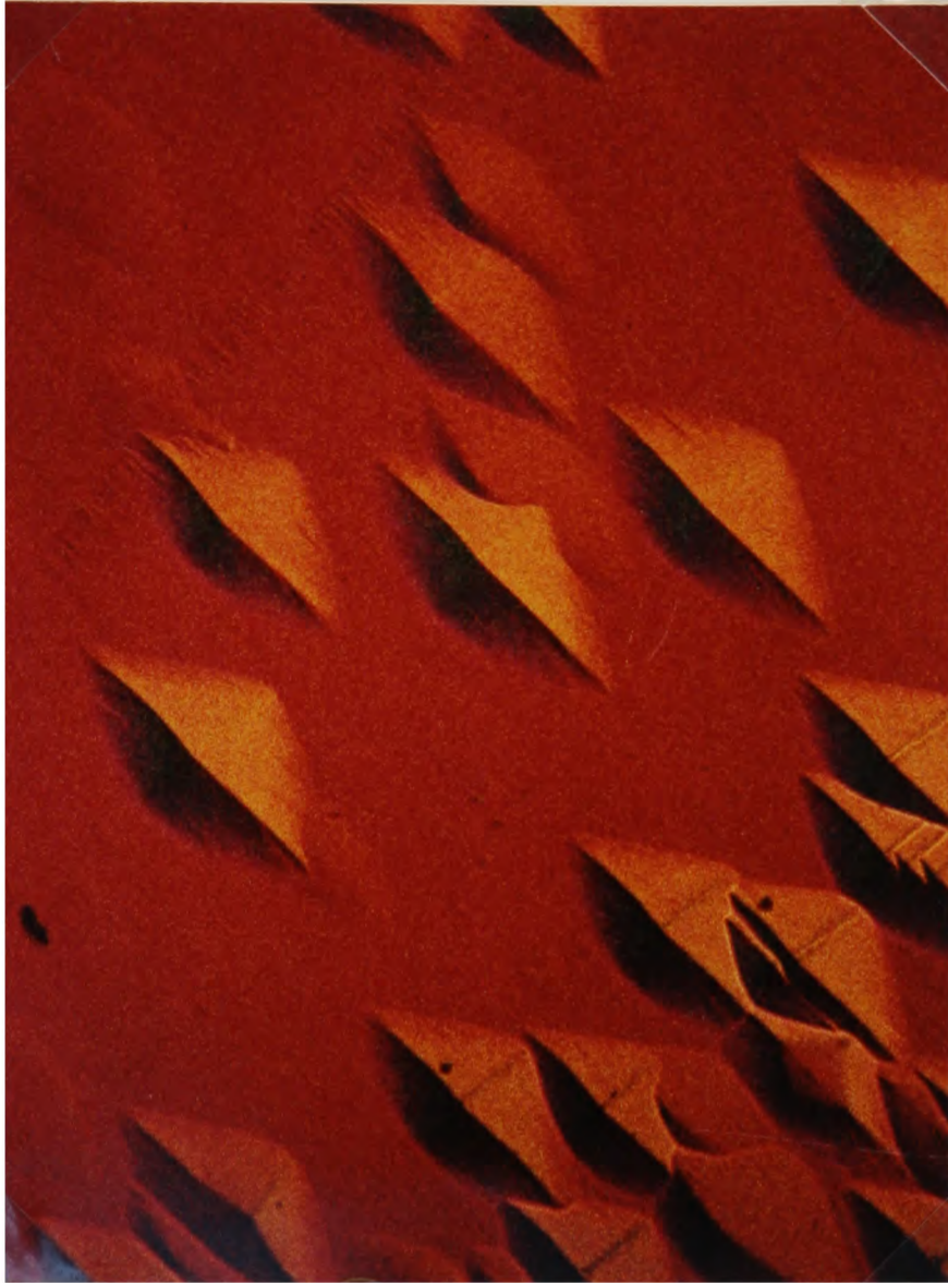
Plate 5. DIC micrograph of a calcite crystal etched in a solution containing 50 mM succinic acid (pH 9.14 - 8.81) and 0.35 M KCl for 10 hours (magnification approximately x200).
