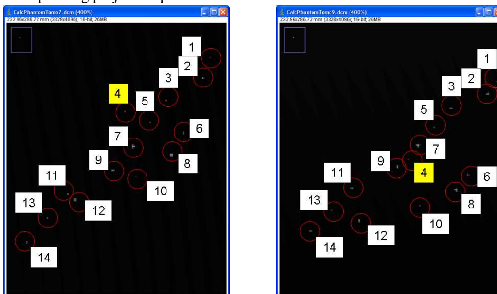
Figure 6.13: The correspondence answer of two DBT views at different angles obtained from the same simulated breast, magnified with a curvilinear cluster of 14 microcalcifications. Left: -0.16^\circ . Right: 5.5^\circ .
