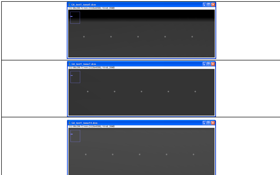
Figure 9.23: DBT views containing a cluster of 5 microcalcifications with different “ b ” values and fixed “ a ” and “ c ” values, generated at -19.98^\circ (Left), -0.16^\circ (Middle), 19.65^\circ (Right).
