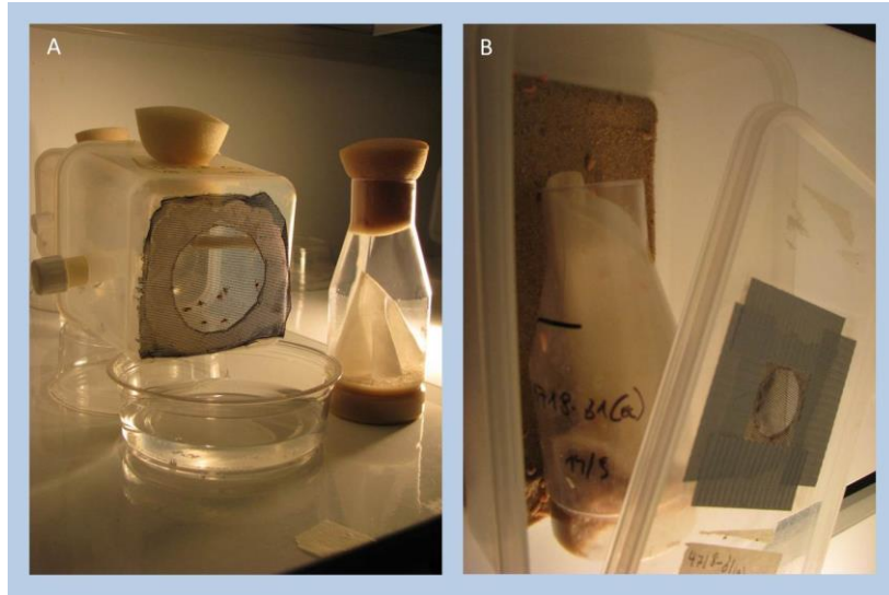
Figure 2.2 Equipment for rearing Mediterranean fruit flies. The Ceratitis capitata rearing cage and bottle with larval food (inside visible folded filter paper with filtered eggs) (A); plastic box
