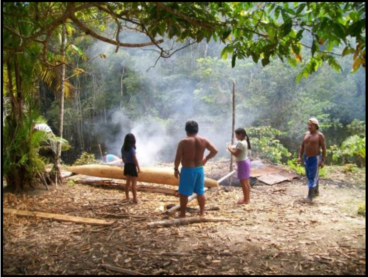
Figure 12: Firing a dug-out canoe to widen its berth. Only men, prepubescent girls and post-menopausal women attend
