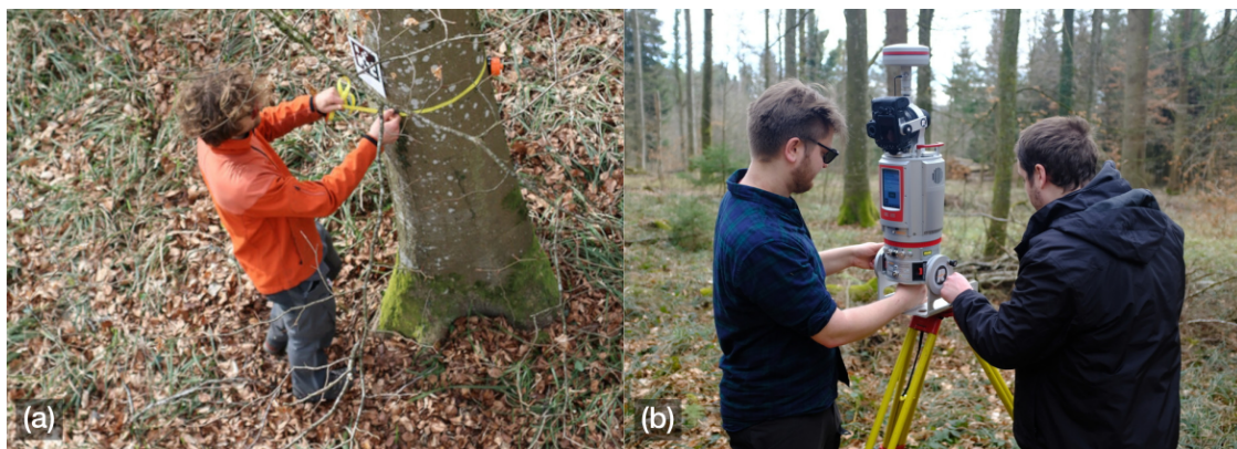
Figure 7.1: (a) Traditional forestry techniques rely on manual measurements using diameter tapes to determine attributes such as the DBH. (b) Nowadays, remote sensing techniques such as TLS provide more accurate measurements in a systematic way. Source: DigiForest EU project, Stein am Rhein Field Trial .
