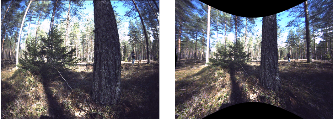
Figure 2.7: Fisheye lens distortion in the Sevensense Core Research sensor. Left: Distorted output before fisheye correction, henceforth displaying curved trees. Right: Undistorted image, correctly displaying the trees standing straight. The empty pixels (black) represent areas that are not observed in the original input; these are introduced to match the specified intrinsics after undistortion.
