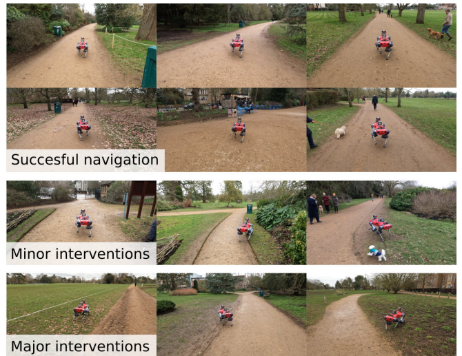
Fig. 11: Kilometer-scale navigation: We deployed our system to learn to segment the footpath of a park after training for a few steps. We executed 3 runs starting from different points in the park: ■ run 1 (0.55 km), ■ run 2 (0.5 km), and ■ run 3 (1.4 km). Minor interventions were applied to guide the robot in intersections; major interventions (★) were required for some areas when the robot miss-classified muddy patches for the path.
