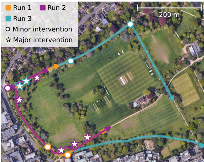
Fig. 11: Kilometer-scale navigation: We deployed our system to learn to segment the footpath of a park after training for a few steps. We executed 3 runs starting from different points in the park: ■ run 1 (0.55 km), ■ run 2 (0.5 km), and ■ run 3 (1.4 km). Minor interventions were applied to guide the robot in intersections; major interventions (★) were required for some areas when the robot miss-classified muddy patches for the path.
