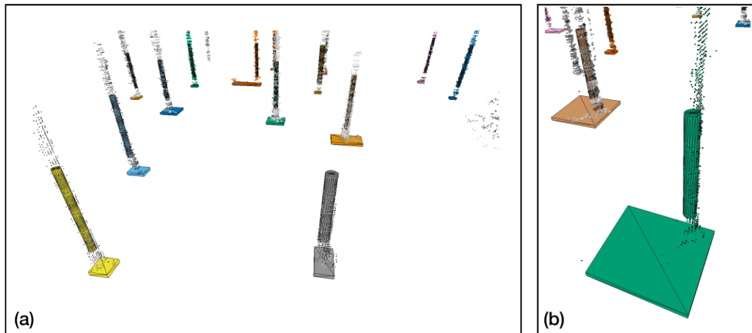
Figure 7.21: Correct cylinder fitting for different payload data. (a) An example of correct detections in one of data payloads. (b) Successful cylinder fitting in spite of the partial observability.
