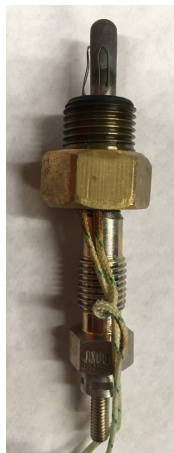
Figure 4.7. The surface pre-ignition sensor adaptor with holes for sensors and glow-plug
