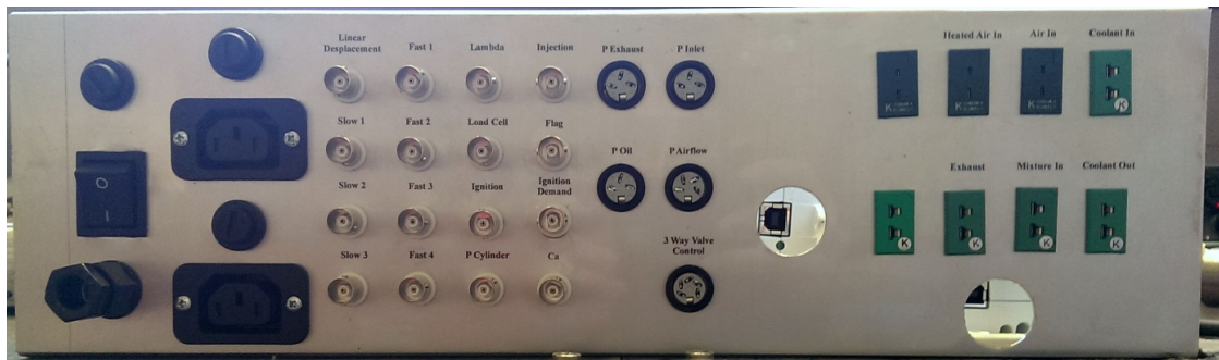
Figure 2.4. Interface control box back panel with clearance holes for DAQ-card cables
