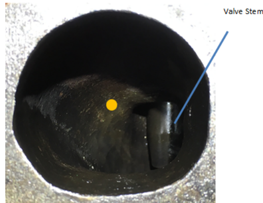
Figure 2.4. Photograph of inlet area. Yellow dot is used to mark the centre point where fuel impinges.
