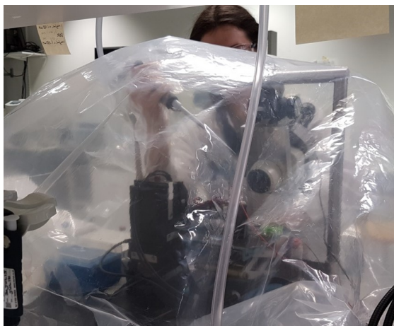
Figure 4.5: Operation of the droplet printer inside in an Atmosbag TM (Sigma-Aldrich) was found to be impracticable. See Section 6.7 .
