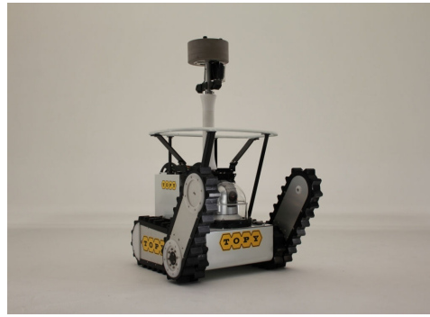
(b) 'Road Runner' robot deployed by Tokyo Electric Power Company (TEPCO) to map the extent of the radioactivity leak. (Source: TOPY Industries, http://www.topy.co.jp )
