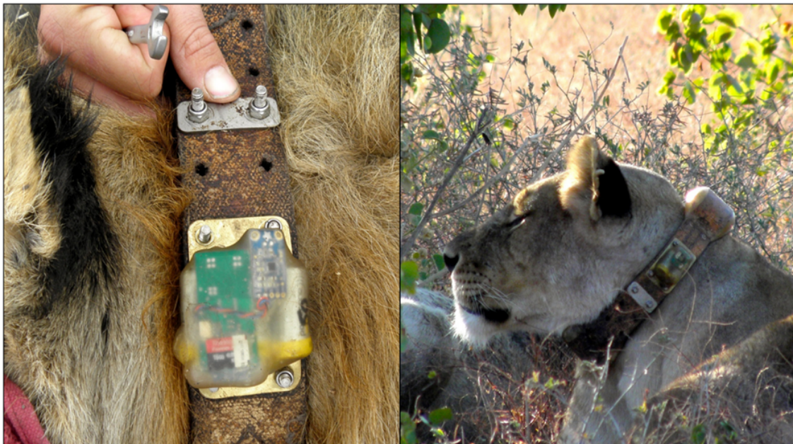
Figure 2.1 Image showing bilogger bolted to a GPS collar fitted to a lioness.
