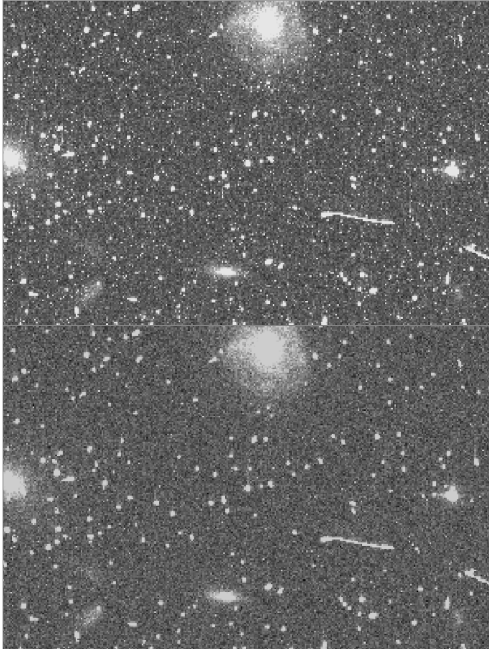
Figure 2.2: Differences between a raw (top) and a f1t frame (bottom) from ACS: the calibrated f1t frame background looks much smoother than that of the uncalibrated raw frame. Cosmic rays still affect the f1t frames, and will be dealt with in successive steps (MULTIDRIZZLE, see text). Both images cover the same area of \sim 14'' \times 10'' .
