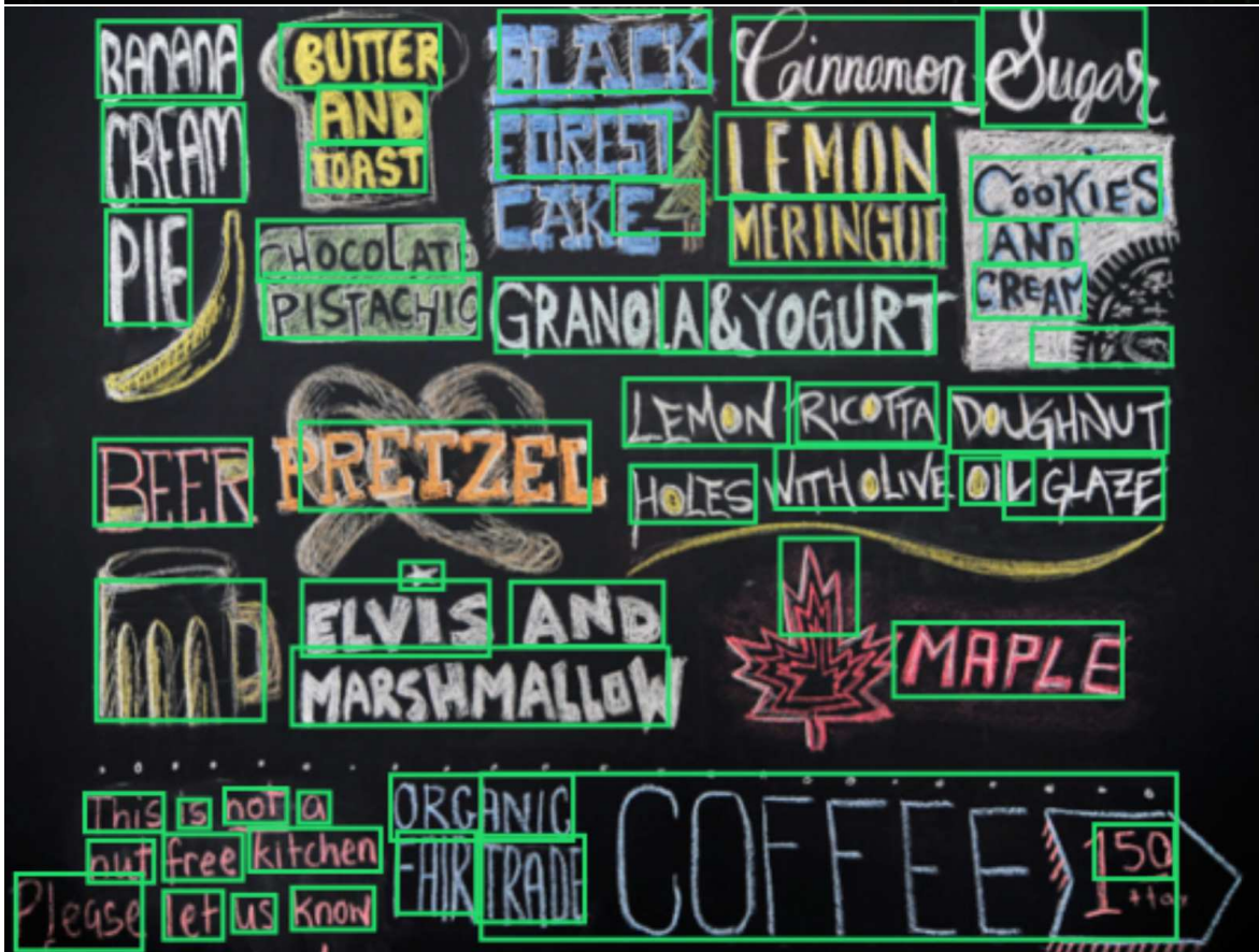
Figure 1.2: Text localisation in the wild. Visualisations of text detections from our detector on two images. Note, in the second image, the method generalises to hand-written text, even when it is trained only on synthetically rendered fonts. View detailed results for these images at our online demo: top , and bottom .
