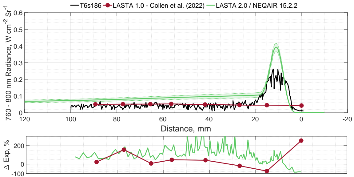
Figure 4.12: Integrated 760 nm - 800 nm radiance profiles for shot T6s186. Dashed lines and shaded region represent \pm 100 \text{ m s}^{-1} perturbations to the shock trajectory
