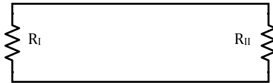
Figure 1.1: Two resistors R_I and R_{II} with resistance R connected using a long non-dissipative transmission line 20 .
