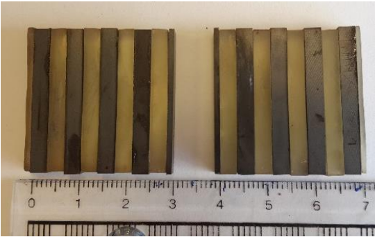
FIG. 6.12. Multilayer tiles comprised of alternating layers of NiZn ferrite bars and epoxy resin with a size of 30 \times 30 \times 4.8 mm.
