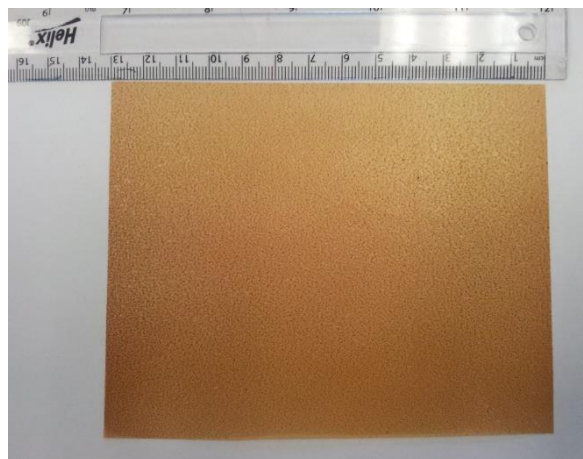
FIG. 5.12. Photographs of 13 \times 13 cm PFA/Fe 3 O 4 (ferrofluid)/PFA nanocomposite films.
