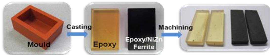
FIG. 3.1. Photographs of the silicone mould, casted epoxy and epoxy-NiZn ferrite composite samples. The samples were subsequently machined into two identical pieces for permittivity and permeability measurements.
