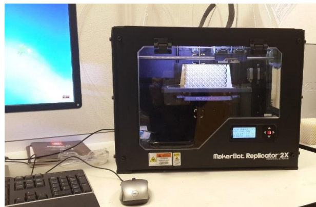
FIG. 3.5. Photograph of the 3D printing, or additive manufacture, setup with 100 \mu\text{m} layer resolution and up to 28.4 \times 15.5 \times 15.2 cm build volume.
