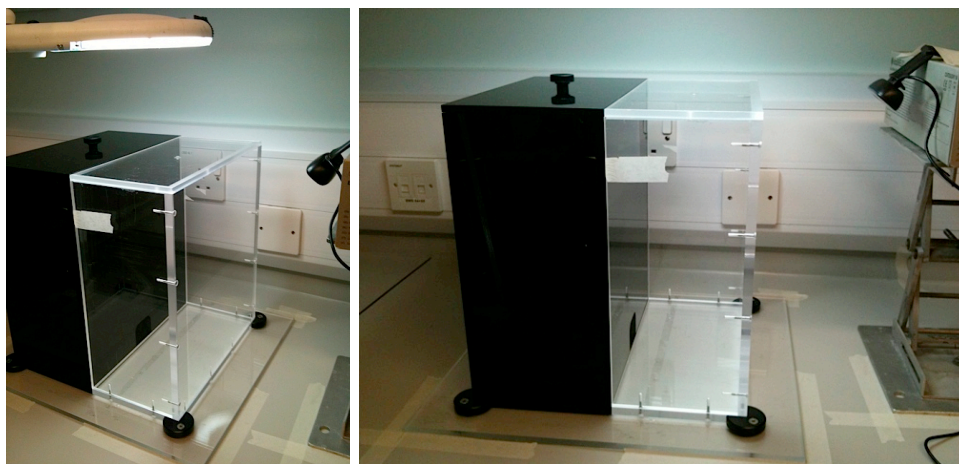
Figure 7.1 Light-Dark Box apparatus Side and corner views of light/dark box used for test of light avoidance behavior to white and UV light in the Opn1sw transgenic model
