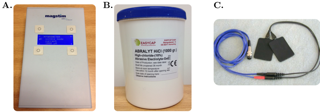
FIGURE 2.1: Components of a tDCS kit. A. Battery operated DC stimulator. B. High Chloride Electrolyte-Gel for the conducting medium between the scalp and electrodes for tDCS in the scanner. C. Rubber electrodes and connecting wires.
