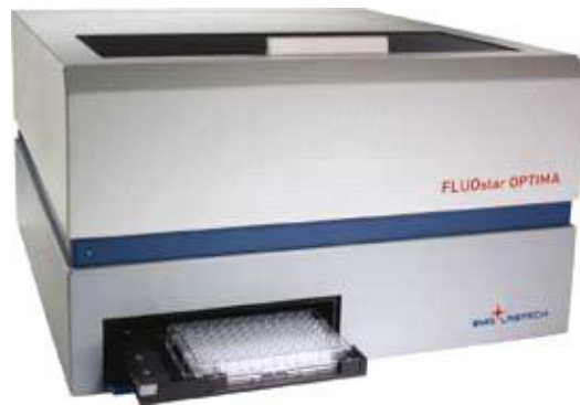
Figure 3.5. FLUOstar OPTIMA fluorescence microplate reader for the evaluation of the metabolic activity of osteoblast cells, using alamarBlue® assay 160 .
