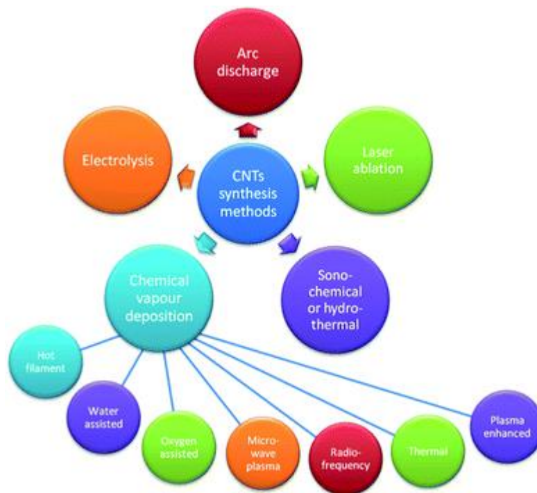
Figure 1.11. Various methods for CNTs synthesis used to date 72 .
