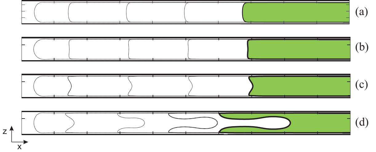
Figure 5.2: Interface evolution in the x-z plane for varying surface tension. The time interval between the plotted interface positions is \delta t = 5 \times 10^4 time-steps in lattice units. The thickness of the cell and the wetting layer are b = 70 and \zeta = 5 respectively in lattice units. Surface tension: (a) \sigma = 9.36 \times 10^{-3} , (b) \sigma = 5.85 \times 10^{-3} , (c) \sigma = 3.51 \times 10^{-3} and (d) \sigma = 2.34 \times 10^{-3} .
