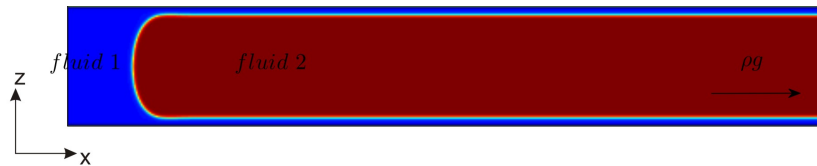
Figure 5.1: Schematic representation of the interface configuration in the x-z plane if the less viscous fluid 1 wets the substrate. The system is initially left to relax until a meniscus is formed and then the body force \rho g is turned on.
