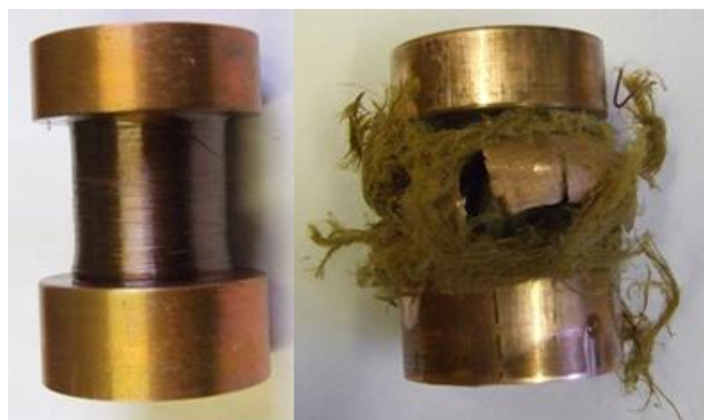
Figure 5.13. A Zylon fibre sample before and after testing.
