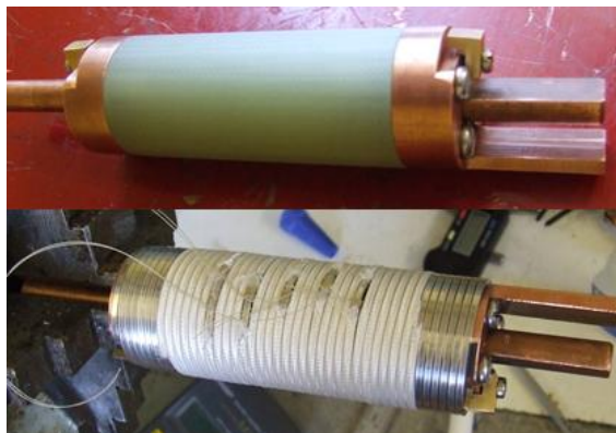
Figure 3.5. The former for the single layer coil and the completed coil constructed for the critical current measurements.
