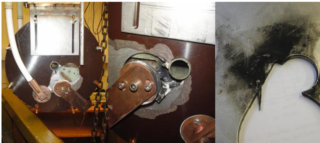
Figure 4.30. Damage caused to both sides of the coil pair during pulse 138 and the spark-erosion of the stainless steel plate.
