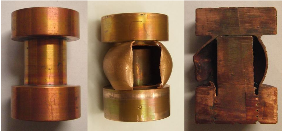
Figure 5.11. Photos showing a new vessel on the left and the final state of two vessels after completion of a run with the entire 3mm vessel in the centre and a cut-away of the 1mm vessel on the right. The solder filled threads are clearly visible at the bottom of the 1mm vessel.
