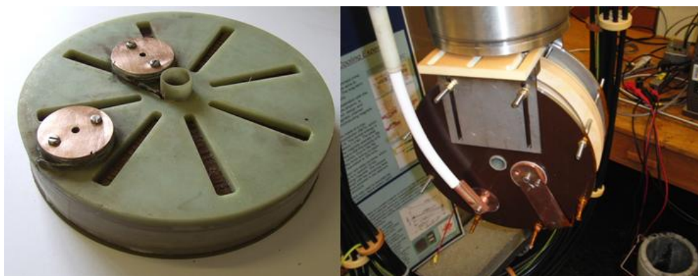
Figure 4.22. Completed coil with wire soldered to current contacts and the completed coil pair mounted on the pulse module with the 6F/45 hanger plate clearly visible.
