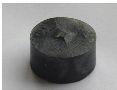
Figure 6.11. The GdBCO single grain sample used in the flux trapping experiments.
