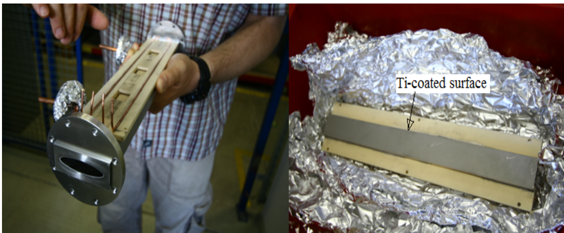
Figure 5.49: Nonlinear pulsed kicker used in Bessy-II (left), Ti-coated ceramic chamber (right).
