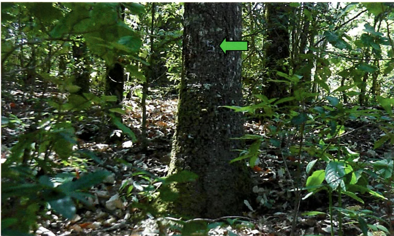
Photo 2.1 Tree indelibly labelled with white water proof silicon paint (green arrow) marked at least 10 cm above the point of dbh measurement.
