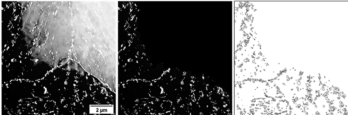
FIGURE 7 Segmentation of the ADF image to isolate individual precipitates, with the metal-matrix excluded.
