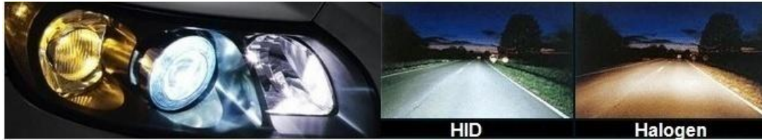
Figure 7. 10. Comparison between Xenon High Intensity Discharge and Halogen headlamp photometric 295
