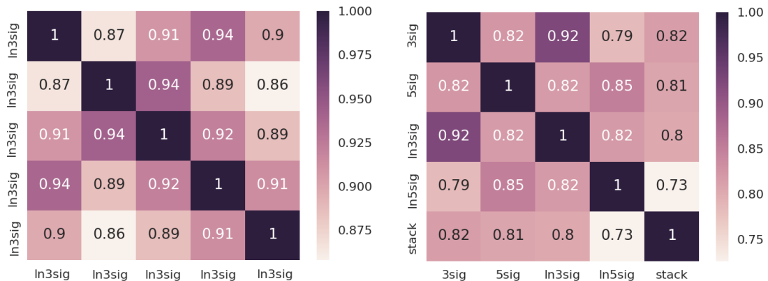
Figure 2.11: Pearson correlation coefficients between the predictions of single CNN (rows, columns) classifiers acting within ensembles using optimal preprocessing (A, left) and varied preprocessing (B, right). Labels denote the preprocessing used for that CNN, with ‘ln’ denoting logarithmic pixel rescaling and ‘Nsig’ denoting the masking threshold used. Configuration A combines five classifiers all using the same optimal preprocessing configuration (logarithmic rescaling and a 3-sigma pixel mask) while configuration B combines five classifiers with varied preprocessing configurations.
