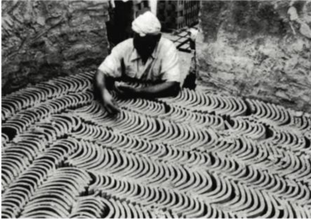
Figure 2.68: Tile-maker at Corigliano loading a kiln. It is possible that the Thracian craftsmen loaded the kilns with tile and brick in a similar manner in order to minimize production time
