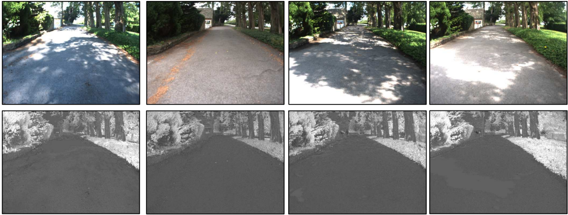
Figure 4.4: Example images taken around our Begbroke Science Park test site, with the raw RGB image shown on top, and the corresponding lighting invariant version shown below. Note how the image transformation is able to significantly reduce the impact of the shadows.
