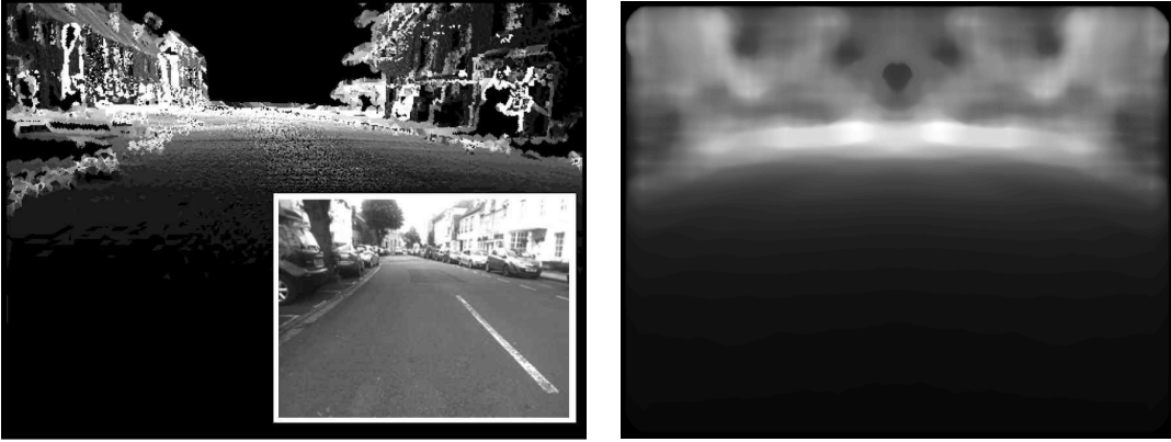
(a) Representative Jacobian image given by Equation (3.10) (i.e., evaluating \partial z^s/\partial \mathbf{x} for each pixel). Camera image provided for reference.
