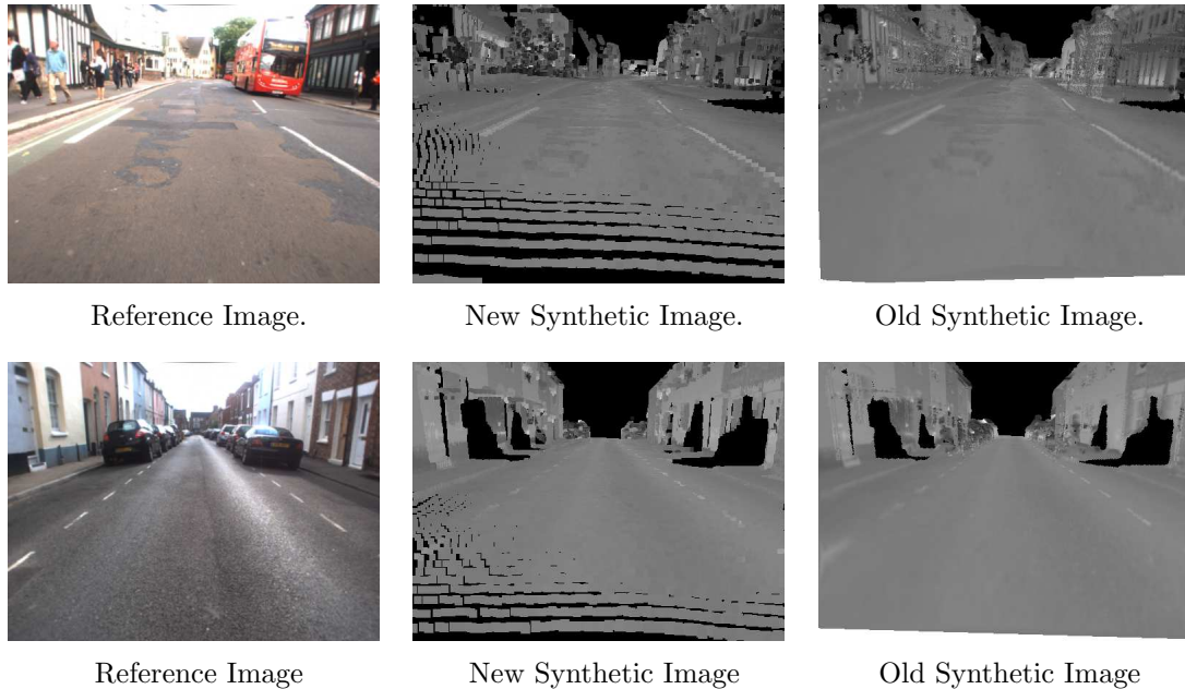
Figure 6.7: Comparison of synthetic images generated using the image-interpolation method described in Chapter 3 versus the new depth-buffered approach. Although the new approach results in a sparser image in the near field, it is significantly faster and allows for 5-10 Hz operation. Additionally, it more accurate in depth since the points are depth ordered. Looking at the interpolated images (far right column), one can see mixed pixel values from the interpolation of the nearest neighbours.
