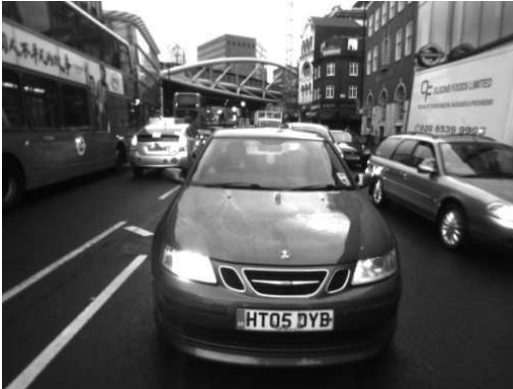
(a) Image taken in central London during the Olympics, where large parts of the scene are occupied by dynamic objects, which can distract and impede egomotion estimation. We present two techniques that leverage knowledge of prior structure to enable robust pose estimation, even in cases where most of the scene is moving.
