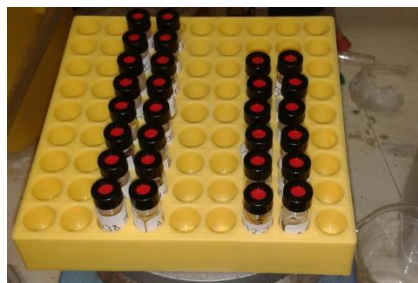
Figure 77 Medium throughput parallel screening setup in the conjugate addition of \text{MeNO}_2 to methyl crotonate and cinnamate.
