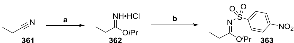
Scheme 73 Synthesis of sulfonylimidate 363 : a) i PrOH, HCl (g), rt, 2 h, 33% yield; b) 4-nitrobenzenesulfonyl chloride, 10 mol% DMAP, \text{NEt}_3 , \text{CH}_2\text{Cl}_2 , rt, 14 h, 72% yield.
