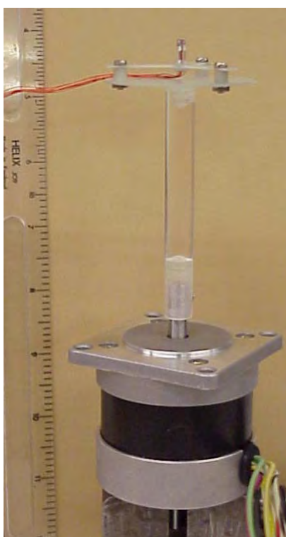
Figure 3.12 – Stepper motor and mount, used to rotate the sensor about a vertical axis (thus changing wind direction). The wind sensor is mounted on the top of the Perspex rod (shown here is an early Beagle 2 wind sensor prototype).
