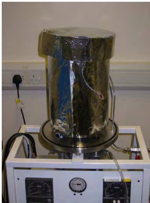
Figure 5.2 – Photograph of cryostat. Visible here is a jacket of multi-layer-insulation (MLI) which surrounds a central chamber. The central chamber contains the isothermal block shown above. The walls of the central chamber, under the MLI jacket, are cooled using a closed-cycle refrigerant loop. The whole assembly shown above is insulated using a vacuum jacket, the O-ring seal of which can be seen on the circular base-plate.
