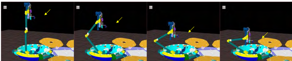
Figure 7.6 – The VERTSCAN positions, like the MEDSCAN and LOWSCAN positions, are intended primarily to make air temperature measurements in the vicinity of the lander. The axis of the wind sensor in these positions is vertical, which may provide observations of updrafts above the hot lander.
