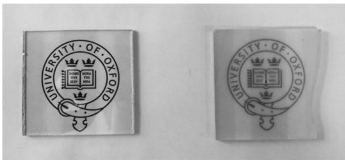
Figure 6.2: (Left) flat \text{TiO}_2 film on an FTO substrate; (Right) macroporous \text{TiO}_2 film.
