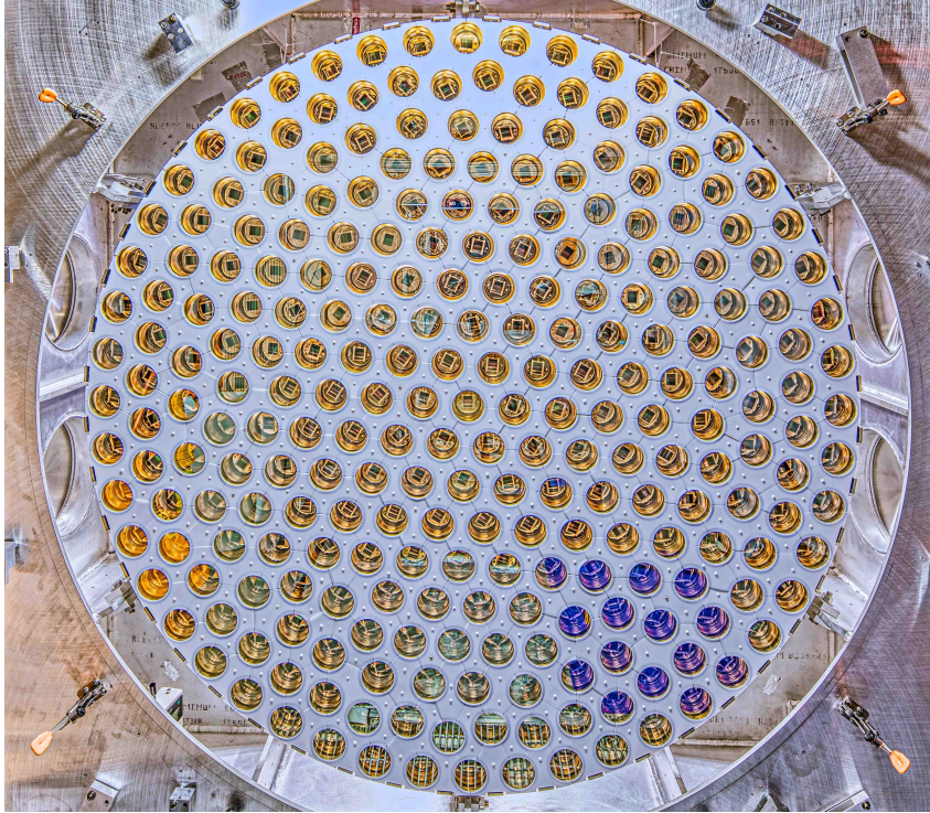
Figure 3.6: The photomultiplier sensors forming the top array within the assembly enclosure. The sensors form a hexagonal structure within the centre, but move to a circular pattern on the outside. This has been optimised to aid in light collection and position reconstruction of events. Photo by Matthew Kapust, Sanford Underground Research Facility. Figure from [101].
