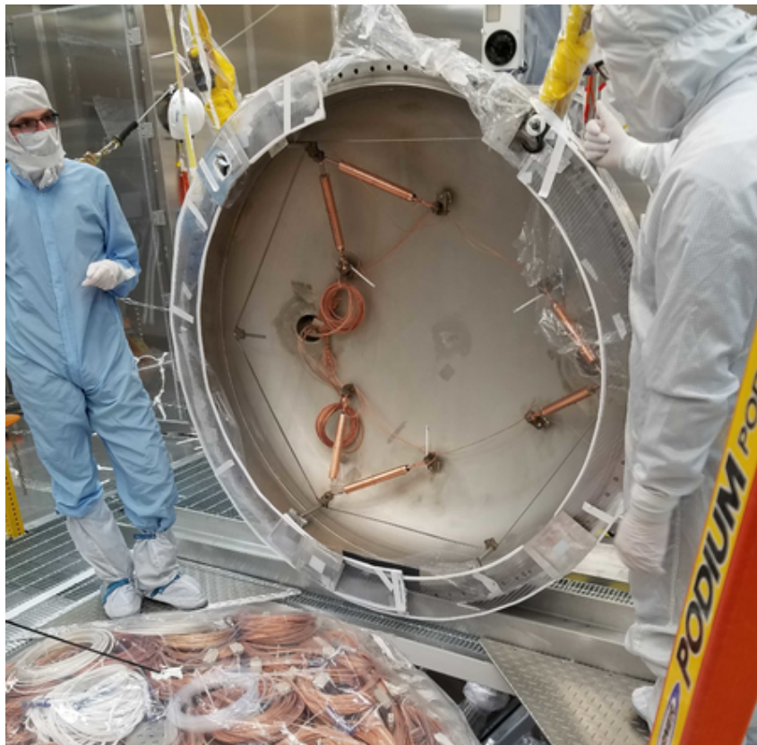
Figure 5.5: The Inner Cryostat Vessel lid (ICV) on its side prior to installation. The main sealing surface is shown here protected with polycarbonate pieces to prevent scratching. The position sensors can be seen within the lid, forming three triangular arrangements. The top array of the TPC (covered in cables) can be seen in the bottom left of this photograph.
