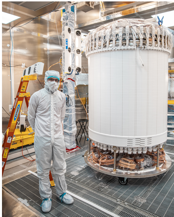
The author with the inner most part of the detector - the TPC field cage and PMT arrays. Credit to Nick Hubbard Sanford Underground Research Facility, July 2019.
