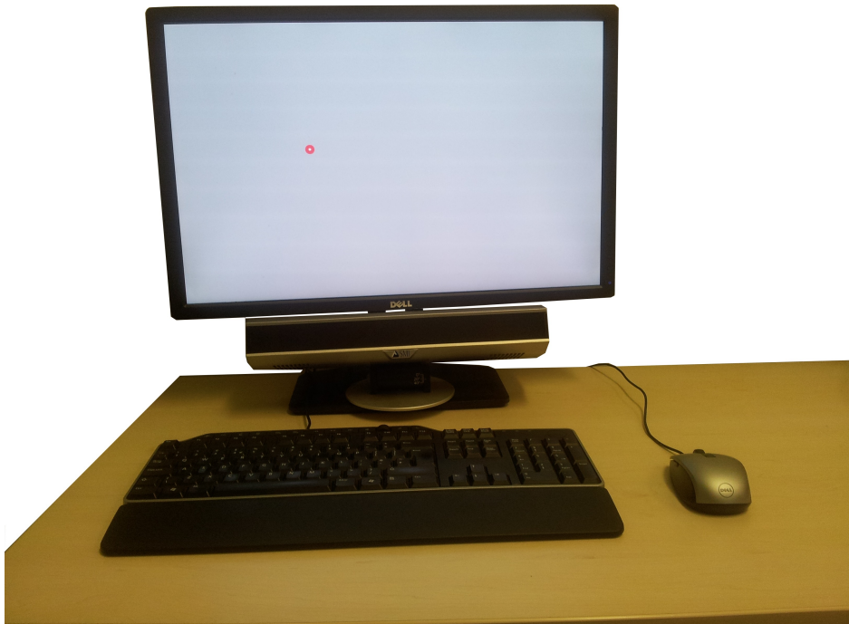
Figure 3.6: Our experimental setup consists of an SMI RED500 gazetracker that determines the user's gaze position on a 24 inch screen with a 1920x1200 resolution
