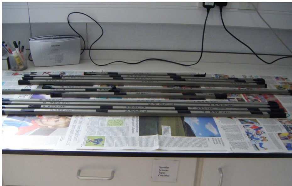
Figure 5.3. Photo of 1 m long U-channels of the M72/25-GC1 core from the Black Sea that were sent to Oxford for cryptotephra investigation.
