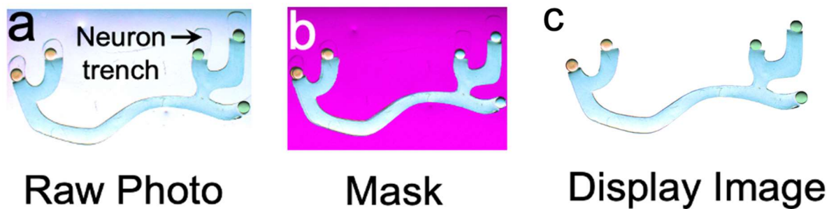
Fig. S29 | Brightfield image processing for display. a , Unprocessed photograph of a synthetic neuron: CM-aR3 droplets (pink, 100 mM MES, 100 mM NaCl, 0.001 % DDM, 0.25 mg mL -1 CM-aR3, pH 6.5), hydrogel axon (blue, 100 mM NaCl, pH 6.5, 2% low gelling agarose) and presynaptic droplets (green, 100 mM NaCl, 50 nM \alpha HL, pH 6.5). b , Background remove selection on Microsoft PowerPoint highlights the background (pink). c , Neuron after background removal generates the display image.
