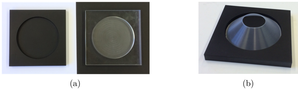
Figure 4.5: Loading docks. (a) Loading docks without specimen on, and (b) loading dock with specimen on.
