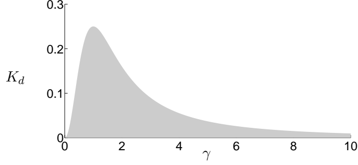
Figure 3.2: The shaded region indicates the parameter sets for which the non-zero equilibrium point, given by Equation (3.21), exists, where \gamma is defined in Equation (3.20).
