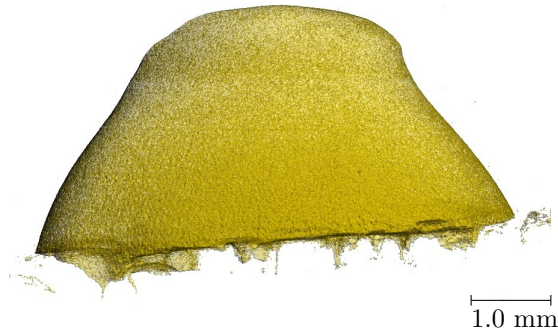
Figure 2.2: \mu CT scan a of sample collagen gel after 14 days of growth showing a roughly hemispherical shape. The shape did not significantly change over the course of the experiment. This gel was produced by seeding 20,000 human mesenchymal stem cells in 300 \mu l of 5 mg/ml of collagen suspension. Courtesy of the ISTM, the University of Keele.
