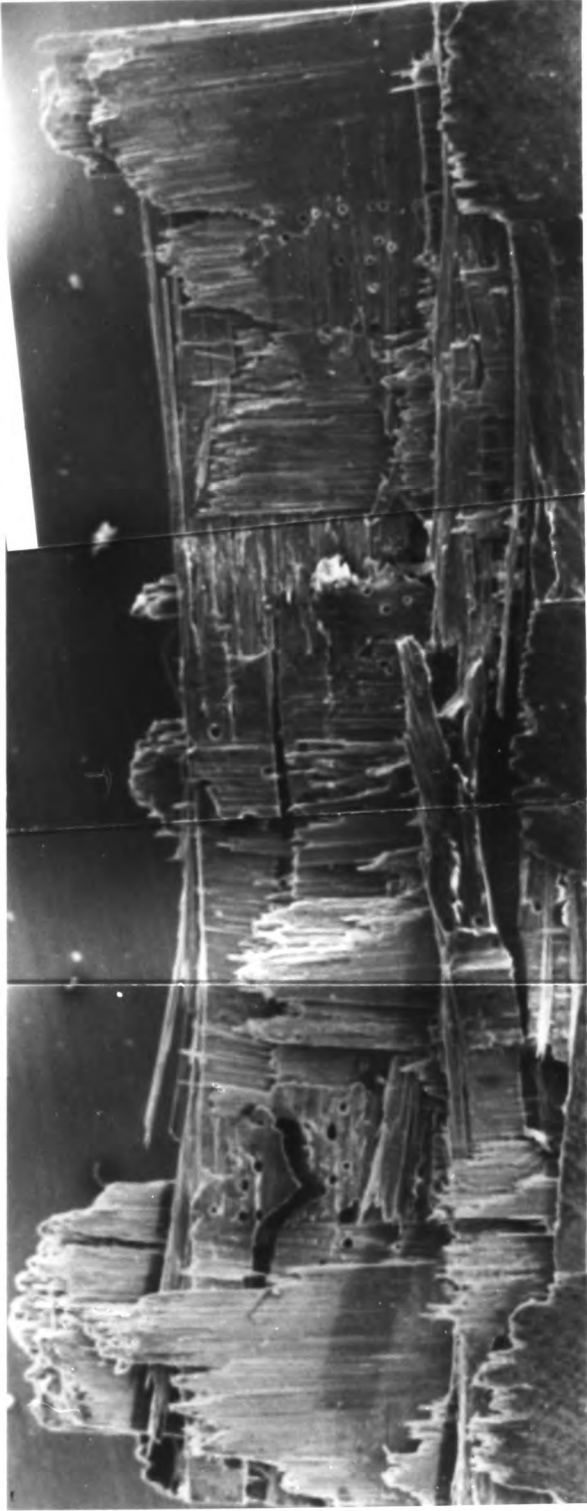
Fig.4.38 SCANNING ELECTRON MICROGRAPH OF FRACTURE REGION OF ALL-CARBON SPECIMEN (x20)
