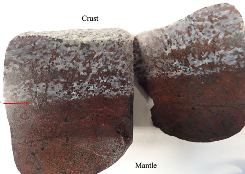
Figure 5. Samples of Moho, showing lower crust gabbro (olivine + clinopyroxene + plagioclase) overlying serpentinised harzburgite (olivine + orthopyroxene ± chrome spinel); Coverack.
