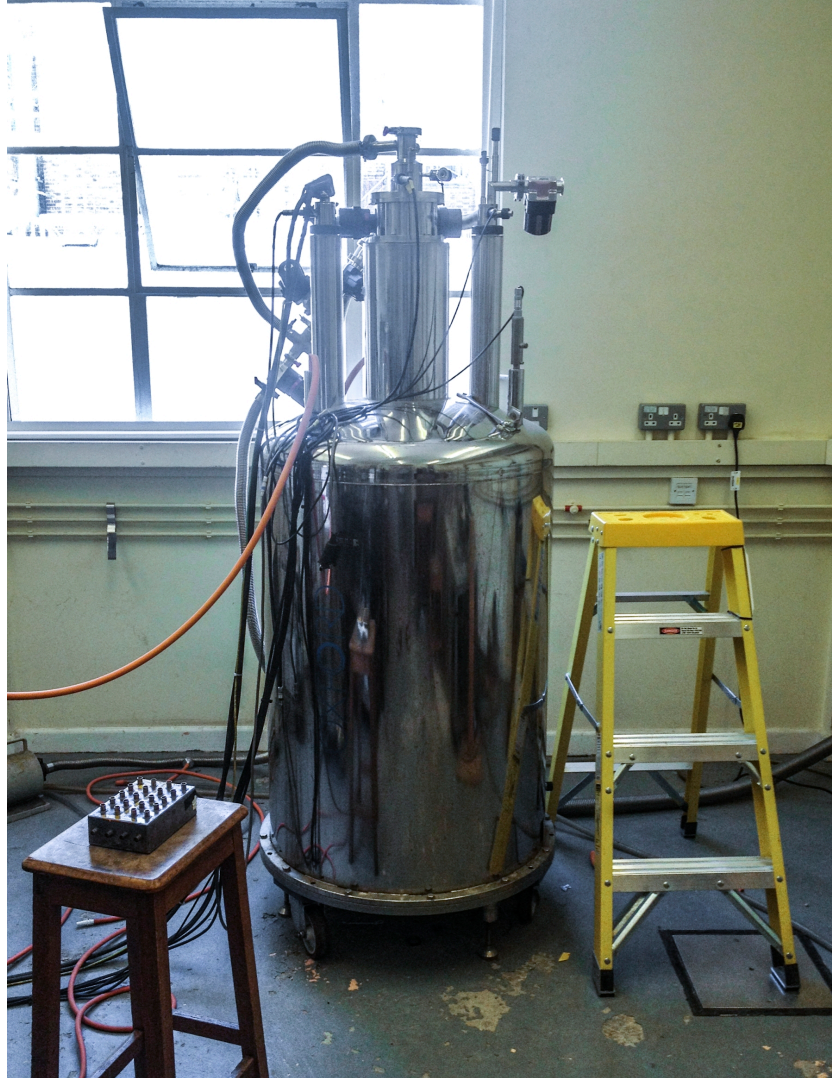
Figure 3.9: Photograph of the 21T superconducting Oxford Instruments Magnet, the primary piece of equipment used in this investigation.
