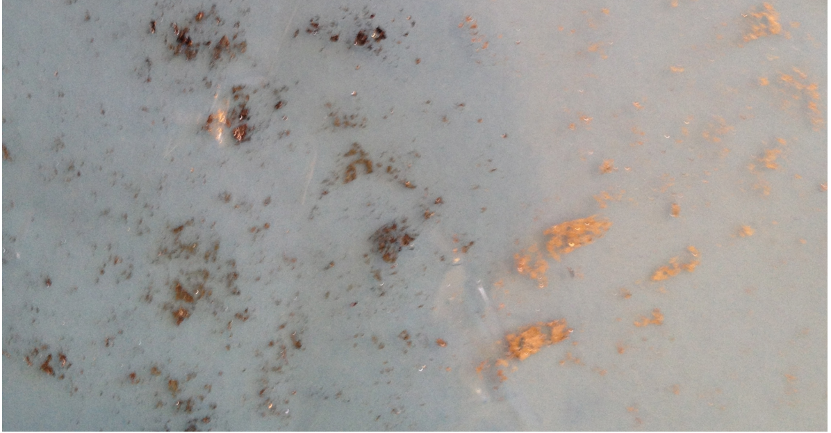
Figure 3.3: Photograph showing the blue Nitto tape commonly used for micro-mechanical exfoliation. Nitto tape is used here, as in the semiconductor industry, since it leaves nearly no residue after removal. In the photograph only the large graphite flakes are visible, coverage of thinner flakes is typically far more complete.
