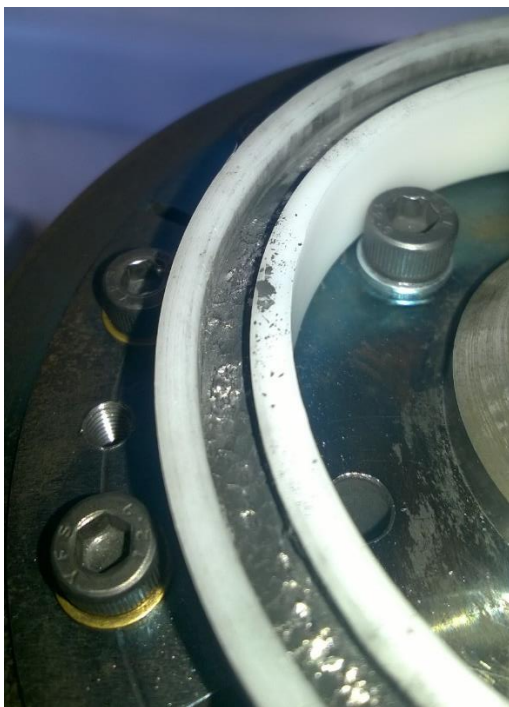
Figure 43: Debris entrapment rings in position, showing the worn surface buried between them.
