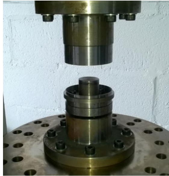
Figure 24: Wear sample mounted on the first wear rig
