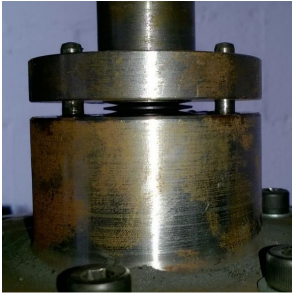
Figure 23: First wear rig: wobble plate, pins and disk spring visible
