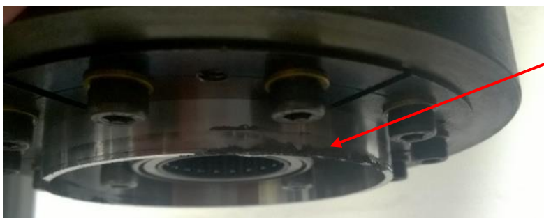
Figure 165: The top sample element showing the accumulation of wear debris above the contact patch
