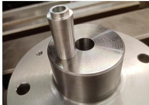
Figure 57: Sample holder with sample as originally produced.
