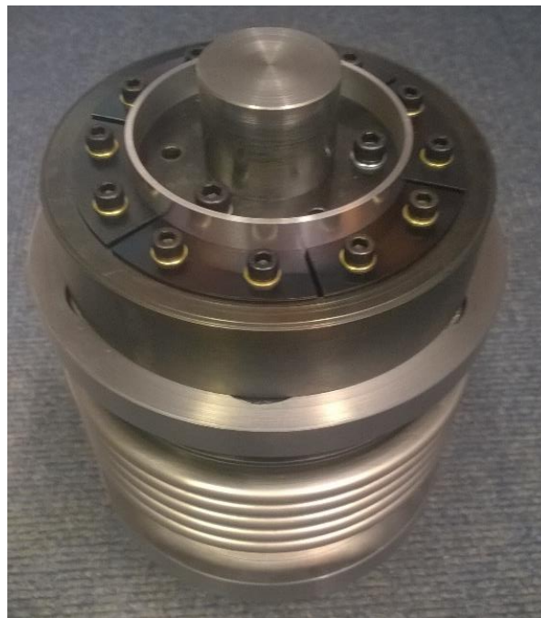
Figure 38: The new wear rig prepared for testing with the Instron loading frame.
