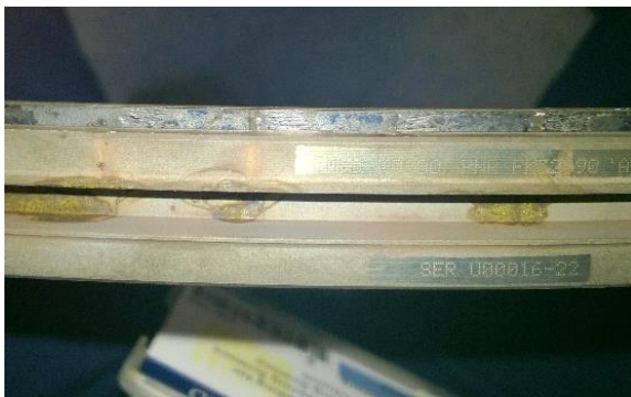
Figure 3: Scuffing marks on the anti-fret liner.
