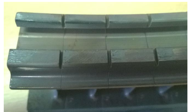
Figure 4: Wear on the compressor blade root.
