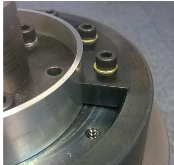
Figure 33: Sample mounted on the sample holder, showing the chucking block.
