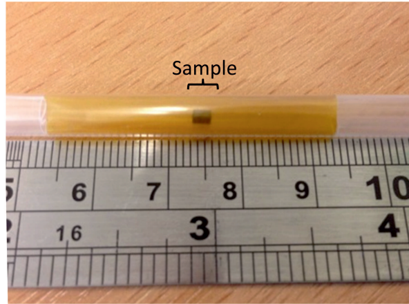
Figure 4.12: Photograph of the solder sample mounted in a straw for MPMS measurement
