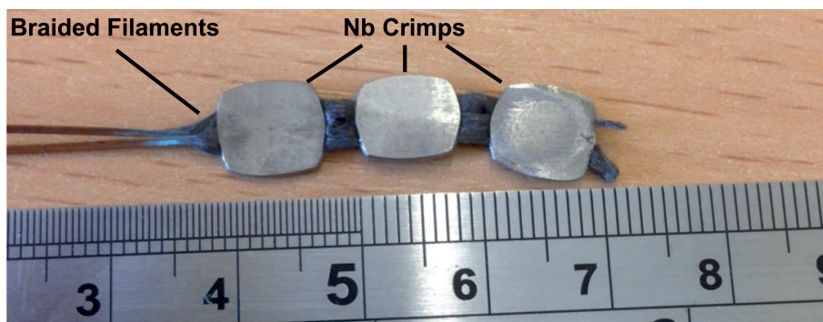
Figure 6.14: Photograph of braided NbTi filaments cold pressed in Nb crimps
