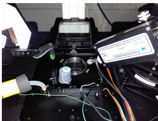
Figure 3.16: Temperature control chamber, eventually not used as it introduced electrical and mechanical noise.
