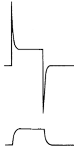
Figure 3.12: Top: Pipette capacitance transients appear in the recorded current trace when a voltage step is held between the electrodes (“Membrane Test”). Bottom: These transients disappear when C_p fast is compensated. Adapted from [114] with permission.
