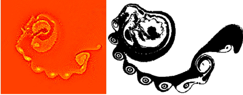
Figure 3.1: The vorticity field after 200000 timesteps obtained using Held et al.’s setup in the SQG code used in this investigation with k_{\max} = 255 resolution (left); and the surface potential temperature (which behaves equivalently to vorticity) plotted by Held et al. (1995) for the same setup (right).
